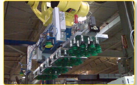
End of Arm Tooling | Zoned vacuum pads for flexibility.
