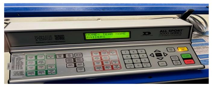
Pull out the plastic card to display the keyboard.
