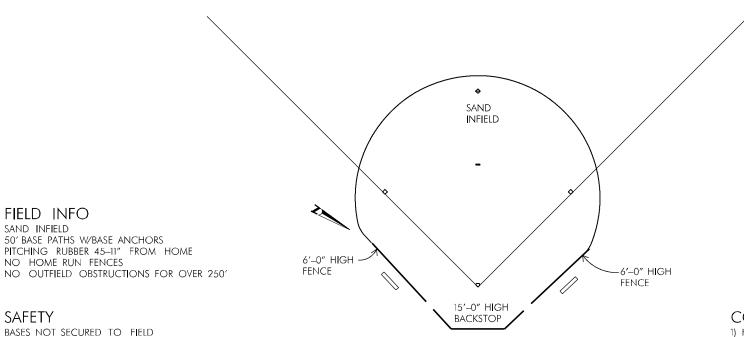
BASES NOT SECURED TO FIELD 15'-0" HIGH BACKSTOP 15'-8" FROM HOME PLATE TO BACKSTOP 19'-6" FOUL TERRITORY ON 1ST BASE SIDE 16'-6" FOUL TERRITORY ON 3RD BASE SIDE CONDITION/IMPROVEMENTS
